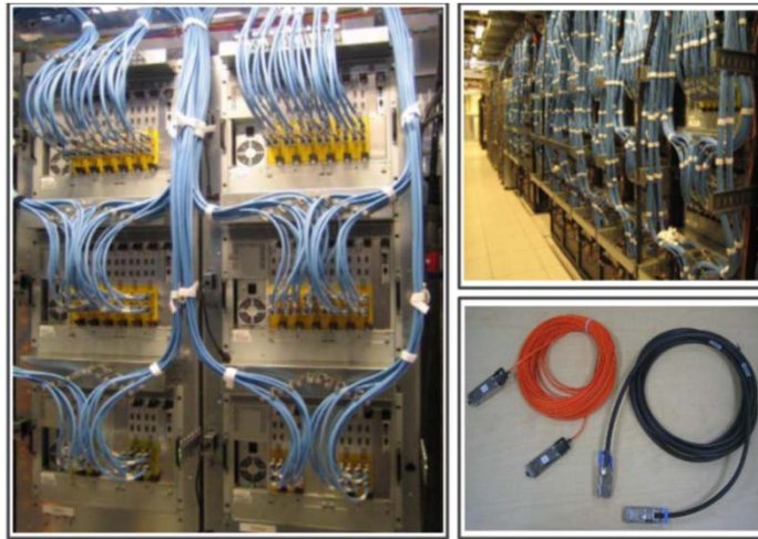
Two Firehose racks (left), each with 3 chassis with bulky CX4 cables from remote racks. The top right figure shows an aisle of cabled racks.
